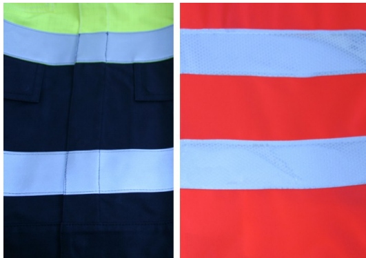
Safety jacket left - all seams stitched conventionally. Safety jacket right - all seams produced by laser welding. © Hohenstein Institute
